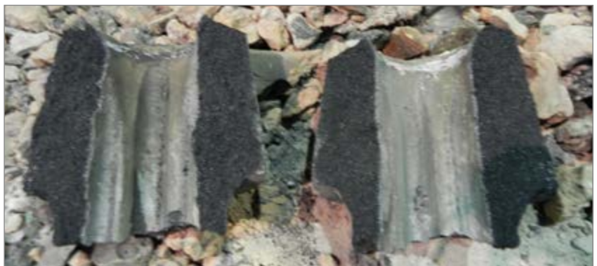
Figure 16. Cross-bore nozzle sectioned after 2 ladle journeys, showing minimum wear of the body material
