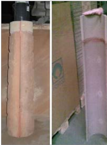
Figure 9. Preheating sheath for KALTEK ladles with small stopper sizes
