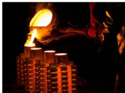
Figure 2. Steel investment casting by a teapot ladle
