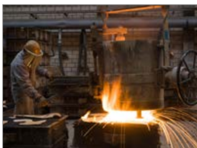
Figure 1. Casting in a steel foundry by monoblock stopper
