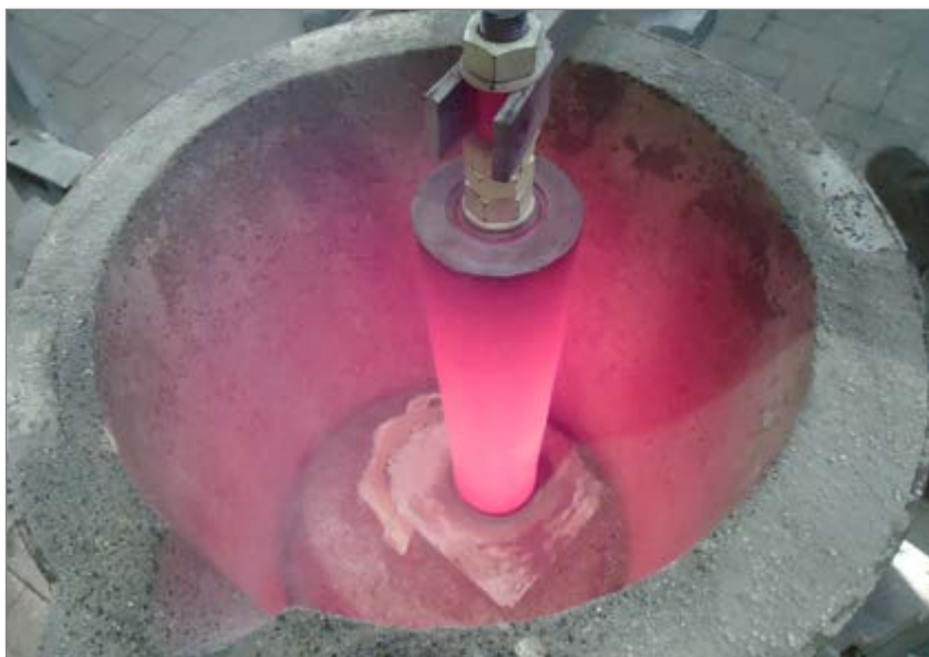
Figure 5. Monoblock stopper after preheating, ready for filling
