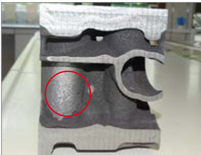
Figure 7. Casting section only after shake out
