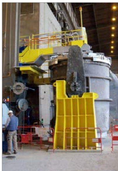
Figure 4. Professional preheating station for large steel casting ladles
