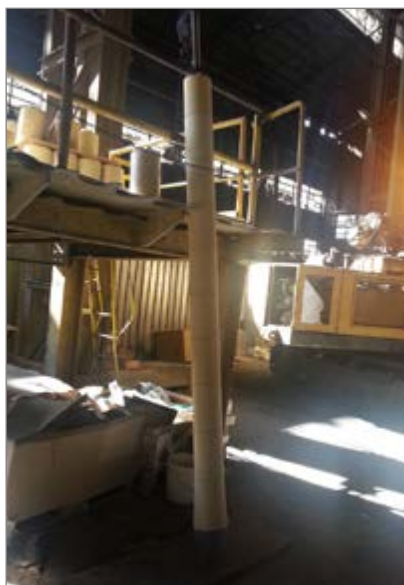
Figure 3. Long assembled stopper in a 35 tonne ladle
