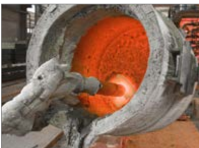
Figure 12. Stopper arm protection by ceramic fibre
