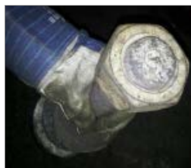
Figure 8. Top: Support rod with vent hole Bottom: DANGER! Blocked vent hole by slag
