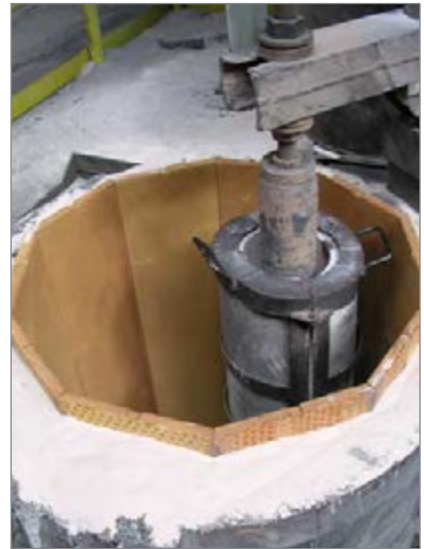
Figure 10. Preheating construction for long monoblock stoppers
