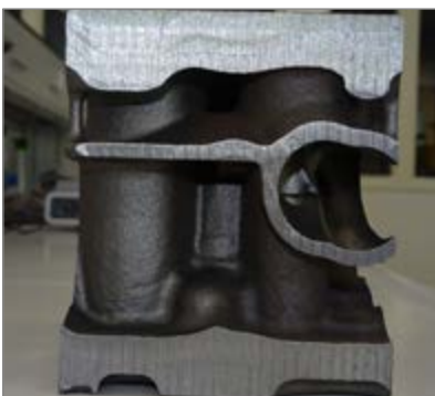
Figure 8. Cast Surface right after shot blasting
